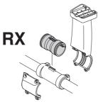
Check that the vibration damping element is undamaged and securely attached.
